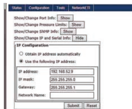
FIGURE 22. IP Configuration Page Showing the Default Settings.
